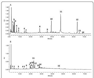
**Figure 1 HPLC chromatograms of** *Qiancao (Rubia cordifolia)* **and** *Qumai (Dianthus superbus)*. Panel A: *Qiancao*; Panel B: *Qumai.* HPLC conditions: column, Agilent Zorbax SB-C $_{18}$  column (150  $\times$  4.6 mm i.d.); flow rate, 1 mL/min; wavelength, 254 nm; mobile phase A, 0.1% formic acid, mobile phase B, acetonitrile. Data was analyzed using Waters Empower software.
